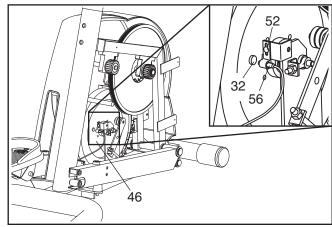
Turn the Flywheel (46) until the Magnet (32) is aligned with the Reed Switch (56) (refer to the inset drawing). Loosen the indicated Screw (52). Slide the Reed Switch slightly closer to the Flywheel, and retighten the Screw. Make sure that the Magnet will not hit the Reed Switch when the Flywheel turns. Repeat until the console displays correct feedback.
